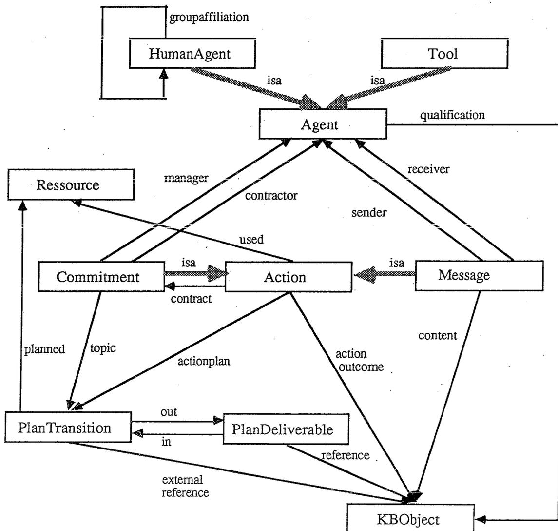
Figure 1: Meta-level Model of Group Problem-Solving in CoNeX
